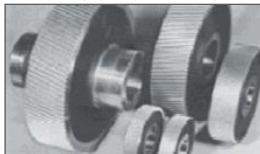
Figure 35 - Steering gears made of class 4 nodular ADI, machined in the ferritic state, with a hardness of 160 HB.
