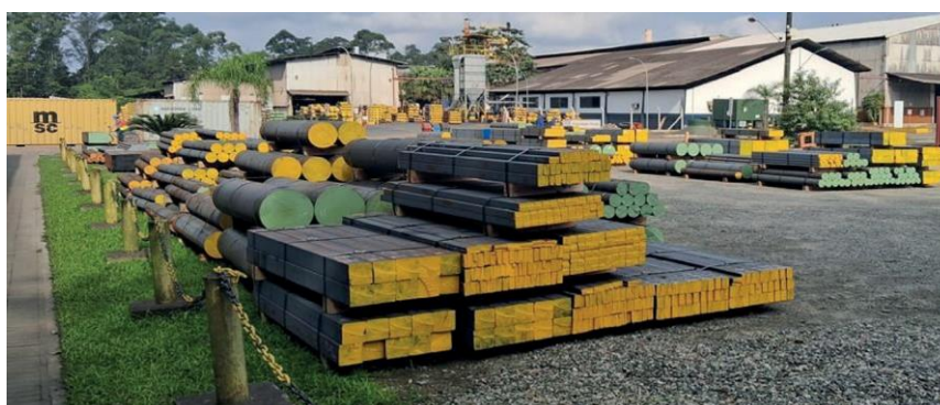
Figure 38 – Identification of bars by Class and Color
