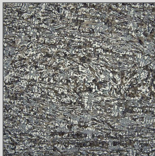
Figure 5b - Typical microstructure at the periphery (VERSABAR® FC 200)
