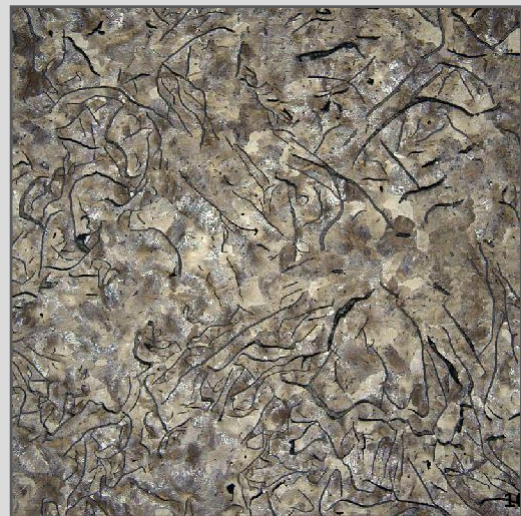
Figure 9b - Typical microstructure at the periphery (VERSABAR® FC 300)
