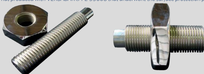
Figure 23 - Shaft and nut produced with VERSABAR® FE 55006 that underwent the surface protection process of chrome plating.
