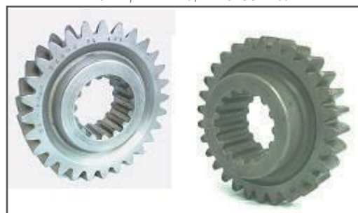
Figure 37 - Examples of gears made of VERSABAR® ADI as a replacement for AISI 8620 steel.
