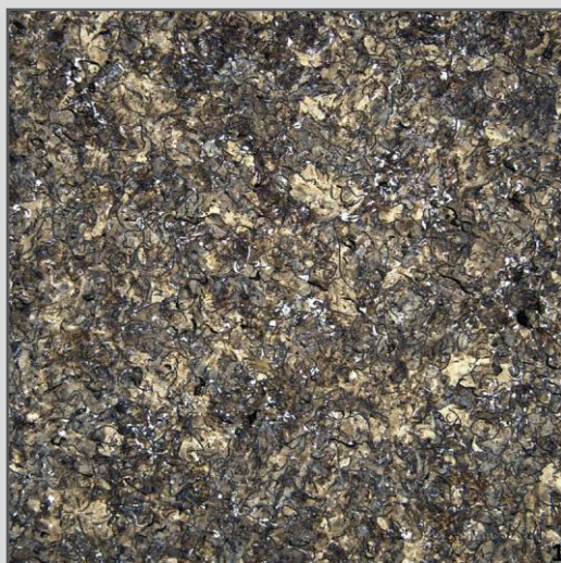
Figure 5a - Typical microstructure at the center (VERSABAR® FC 200)
