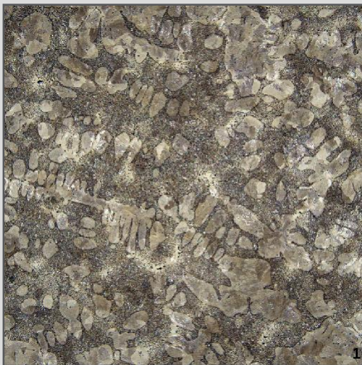
Figure 9a - Typical microstructure at the center (VERSABAR® FC 300)
