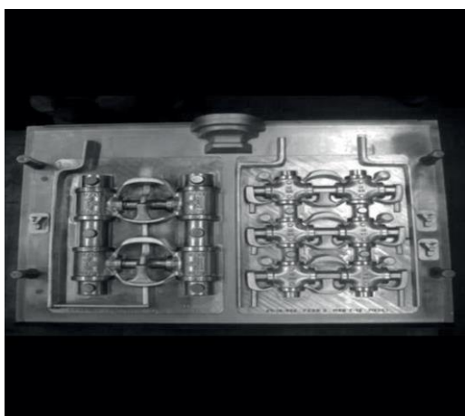
Figure 32a: Green sand molding tooling with VERSABAR® WRI
